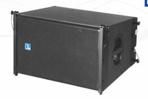
The MLA112 is a small and medium scale line array loudspeaker for long throw distance scale sound reinforcement, fitted with one 12" neodymium LF driver and two 1" neodymium HF driver coupled to a patent line array horn,made of high quality plywood with polyurea waterproof paint. All rigging parts are made of aluminium alloy.
